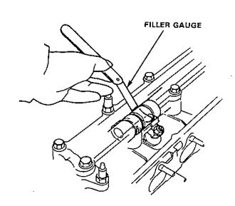
Rotate the crankshaft 180 ° counterclockwise (campulley turns 90°). The "UP" mark should be on the exhaust side. Adjust valve on No.3 cylinder.
