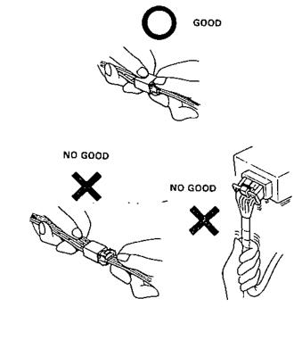
Place the plastic cover over the mating connector after reconnecting. Also check that the cover is not distorted.
