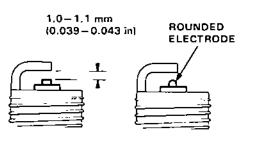
5. Adjust the gap with a suitable gapping tool,
