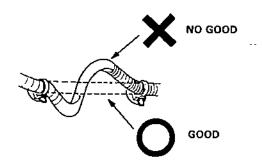
Protect wires and harnesses with a tape or a tube if they are in contact with a sharp edge or corner.
