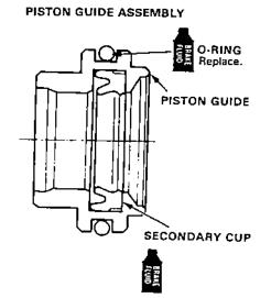
Make sure that the primary piston assembly and secondary piston assembly are in good condition.
