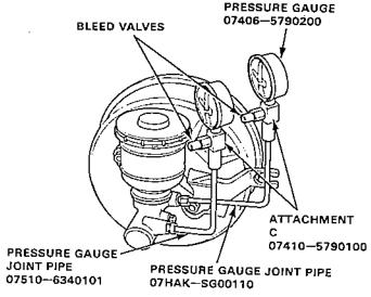
Depress the brake pedal with a 200 N (20 kg, 44 lbs) 5. of pressure. The following pressures should be observed at the pressure gauges in each vacuum.
