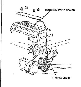
Adjust ignition timing, if necessary, to the following specifications: Ignition Timing:
