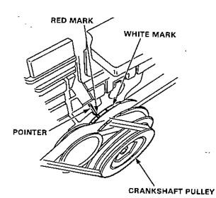
Adjust as necessary by loosening the distributor adjusting bolts, and turn the distributor housing counter clockwise to advance the timing, or clockwise to retard the timing.
