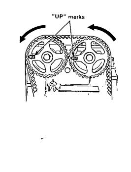
Rotate the crankshaft 180° counterclockwise to bring No.4 piston to TDC. Both TDC grooves are once again visible. Adjust valves on No.4 cylinder.
