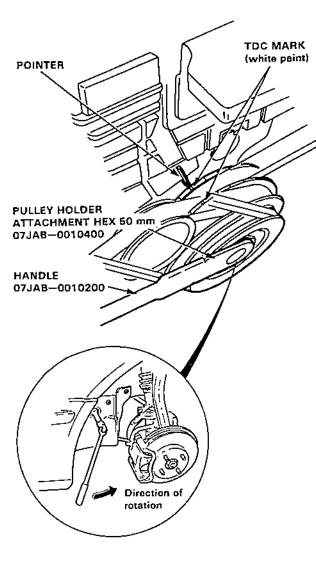
NOTE: If the pully bolt loosens while turning the crank, retorque it to 120 N·m(12.0 kg-m, 87 lb-ft).
