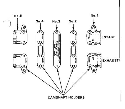
Set the camshaft folders and camshaft holder pipes, then tighten temporaly the bolts.
