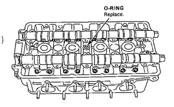
Apply liquid gasket to the head mating surfaces of the No.1 and No.5 camshaft holders, then install them, along with the No.2, 3 and 4.
