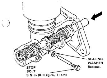
6. Press the secondary piston in and install the new snap ring.
