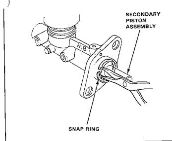
Remove the stop bolt while pushing in the secondary piston assembly.
