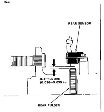
Measure air gap between the sensor and pulser all the way around while rotating the driveshaft by hand.
