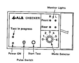
5. With the transmission in neutral, rotate each wheel briskly (one revolution per second) by hand and confirm that its respective monitor light on the checker blinks as the wheel rotares.
