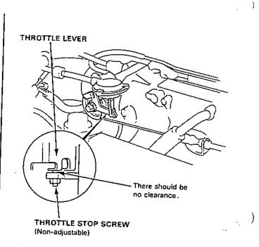
Replace the throttle body if there is excessive play in the throttle valve shaft or if the shaft is binding or sticking.
