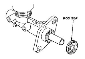
Push the secondary piston assembly, then remove the snap ring.
