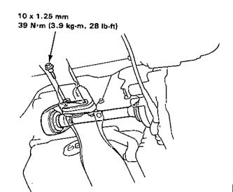
Lower the bearing support close to the steering gearbox and remove the intermediate shaft from the differential.
