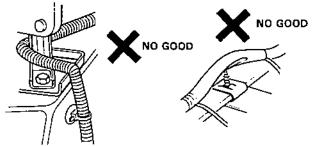
Route harnesses so they are not pulled taut or stackened excessively.
