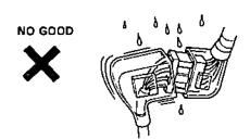
Before connecting connectors, check to see that the terminals are in place and not bent or distorted.
