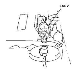
Check idling in no-load conditions in which the headlights, blower fan, rear defogger, cooling fan, and air conditioner are not operating.
