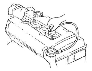
Compression pressure: Standard (new): 1,275 kPa (13.0 kg/cm<sup>2</sup>, 185 psi) at 250 min<sup>-1</sup> (rpm) 932 kPa (9.5 kg/cm<sup>2</sup>, 135 psi) Limit: at 250 min<sup>-1</sup> (rpm) Difference between cylinders: 169 kPa (2.0 kg/cm<sup>2</sup>, 28 psi)
