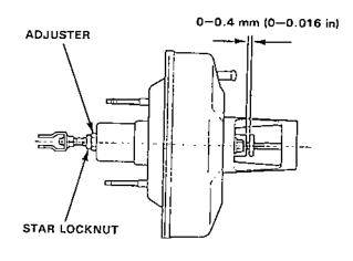
NOTE: If the clearance between the gauge body and adjusting nut is 0 mm, the pushrod-to-piston clearance is 0.4 mm. If the clearance between the gauge body and adjusting nut is 0.4 mm, the pushrod-to-piston clearance is 0 mm.
