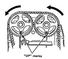
Rotate the crankshaft 180° counterclockwise to bring No.2 piston TDC. The "UP" mark should be on the intake side. Adjust valves on No.2 cylinder.
