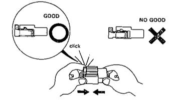
Before connecting, check each connector cover for damage. Also make sure that the female connector is tight and not loosened from the previous use.
