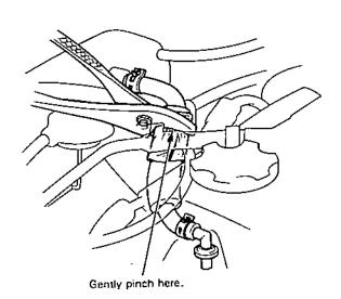
If there is no clicking sound, check the PCV valve grommet for cracks or damage. If the grommet is OK, replace the PCV valve and recheck.
